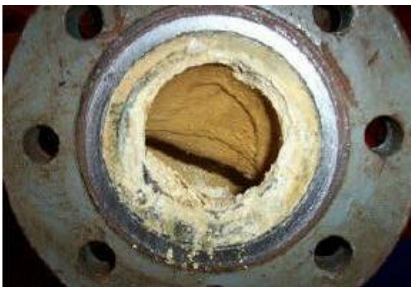
Oil control valve after three months without magnetic fluid conditioners installed
