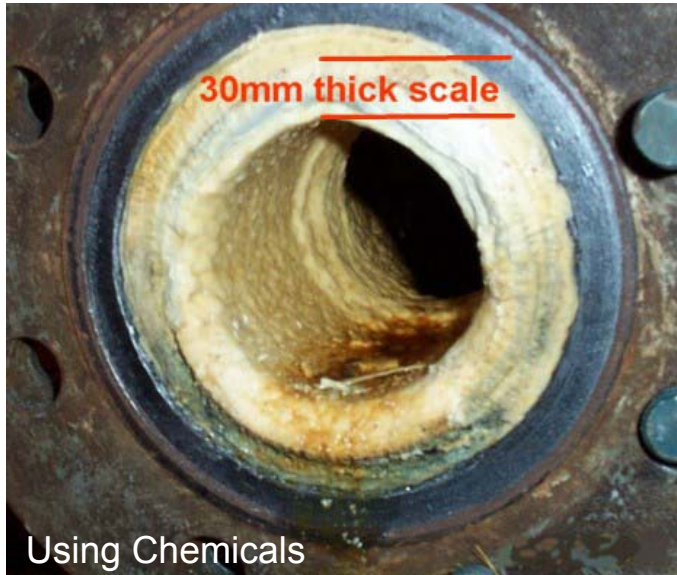
After 3 months using chemical "scale inhibitors"
